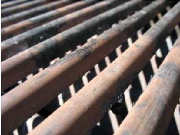
Of interest relative to the case study is that the two cleaners used by the Insured both contained "oxalic acid". This substance functions as a de-rusting agent by preferentially forming an "oxalate" with rusted iron, displacing ("precipitating") the rust and exposing the underlying bare metal. The use of this substance, followed by abrasion, allows the re-formation of a passivated, corrosion resistance surface on the stainless steel.
